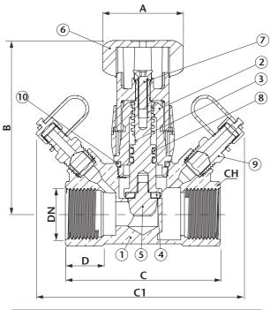
Technical Data 25 Bar Max Pressure -10°C to +120°C **Working Temperature**
