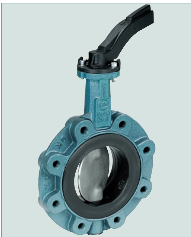
Lug type butterfly valve with threaded holes. This type enables the one-sided lugging of pipes.
