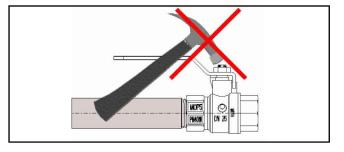
The valve or connecting pipes should not be forced into position
