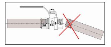
The connecting pipes should be on the correct perpendicular axis
