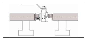
The connecting pipe should be well supported to avoid bending the valve
