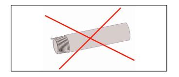
The threaded ends of the pipes should be free from burrs
