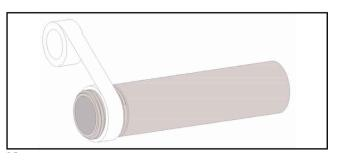
The screwed connections should be made using the minimum amount of PTFE tape
