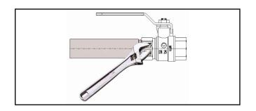
The valve should be held in position with a spanner while the connecting pipes are screwed in
