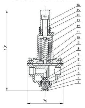
Fitted with standard Pilot Valve 0.70 to 12.00 Bar (10 to 175 PSI) Factory set to 3.5 Bar (50 PSI)
