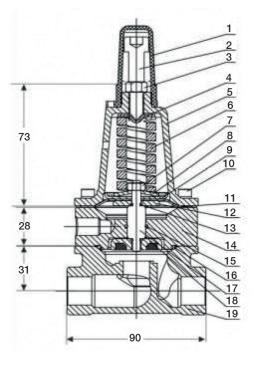
Fitted with standard Pilot Valve 0.70 to 12.00 Bar (10 to 175 PSI)
