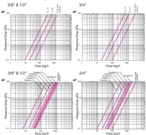
1) Unscrew the cap (or manual handle), tighten the nut clockwise to the limit and identify notch's position. 2) Unscrew the nut to the chosen setting position according to the chart above.
