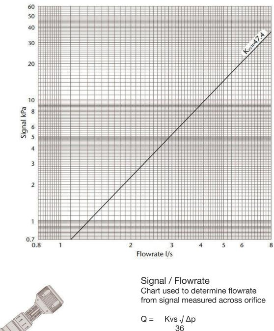
36 Where Q = Flowrate I/s Δp = Signal kPa Kvs = Signal Co-efficient
