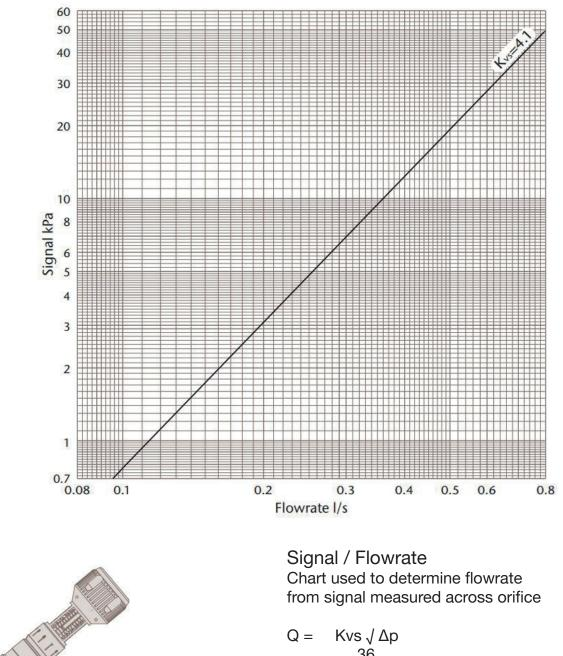
36Where Q = Flowrate I/s  $\Delta p$  = Signal kPa Kvs = Signal Co-efficient
