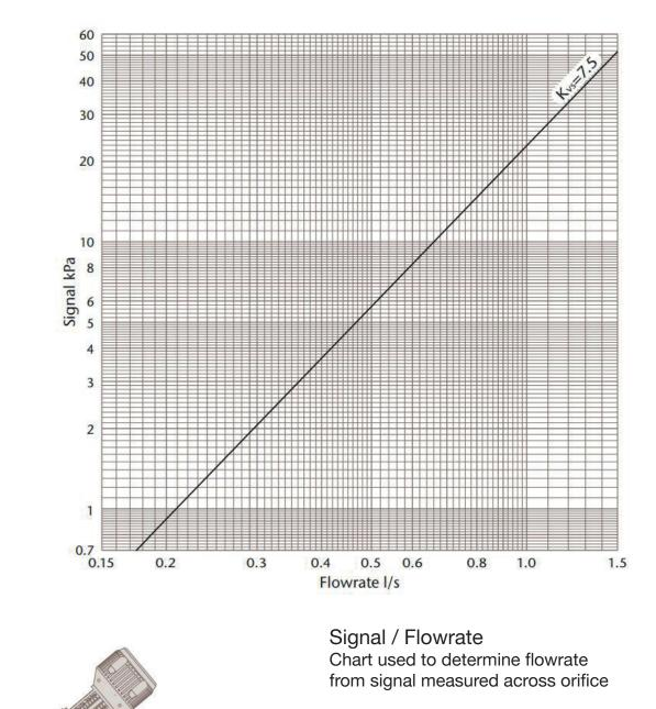
Q = Kvs√Δp 36 Where Q = Flowrate I/s Δp = Signal kPa Kvs = Signal Co-efficient
