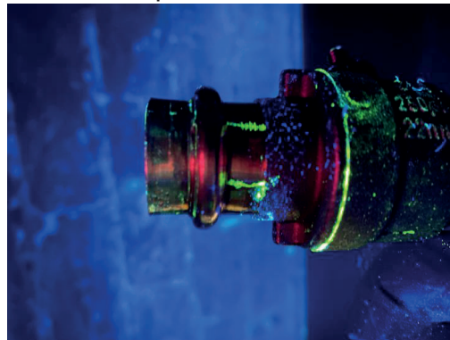
General View - highlighted by fluorescent penetrant
