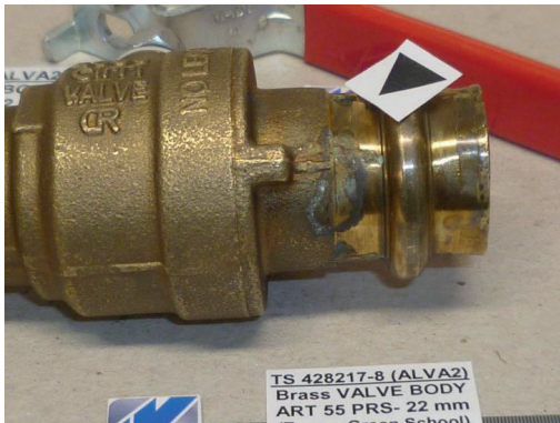
General View of Cracked Area
