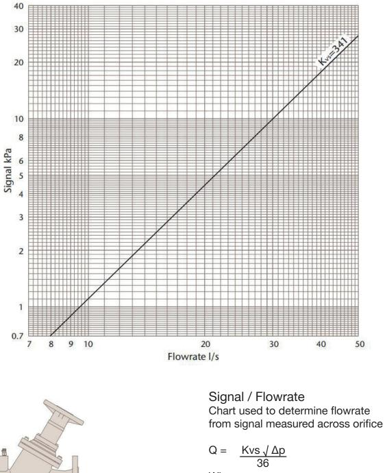
Where Q = Flowrate I/s  $\Delta p$  = Signal kPa Kvs = Signal Co-efficient
