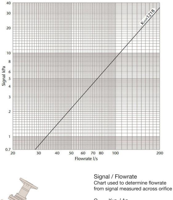
$Q = \frac{Kvs \sqrt{\Delta p}}{36}$ Where Q = Flowrate I/s $\Delta p = Signal kPa$ Kvs = Signal Co-efficient
