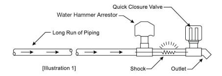
When a unit of equipment is located at the remote end of a long run of piping, the Albion Valves (UK) Ltd Water Hammer Arrestor should be placed as close to the point of valve closure as possible. At this location, the Water Hammer Arrestor will control any developed energy and prevent shock waves from surging through the piping system (Illustration 1).
