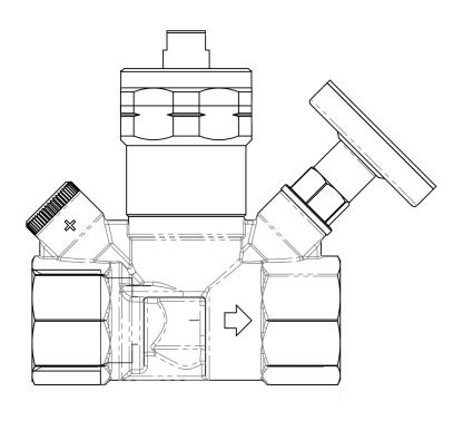
$\begin{array}{lll} \textbf{Pressure Rating} & 25 \ \text{Bar} \\ \textbf{Operating Temperature} & -10 \ \text{^{\circ}C} - 90 \ \text{^{\circ}C} \\ \textbf{Temperature Regulating Range} & 40 \ \text{^{\circ}C} - 60 \ \text{^{\circ}C} \\ \textbf{Anti-Legionella Disinfectant Temperature} & 70 \ \text{^{\circ}C} \\ \textbf{Threads} & \text{ISO 7/1 Rp} \\ \end{array}$
