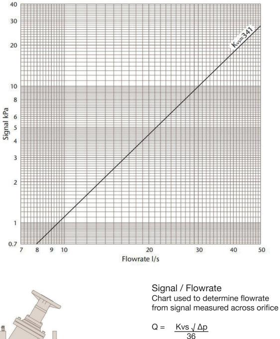
Where Q = Flowrate I/s Δp = Signal kPa Kvs = Signal Co-efficient
