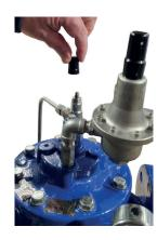
Remove the cap to reveal the adjustment screw
